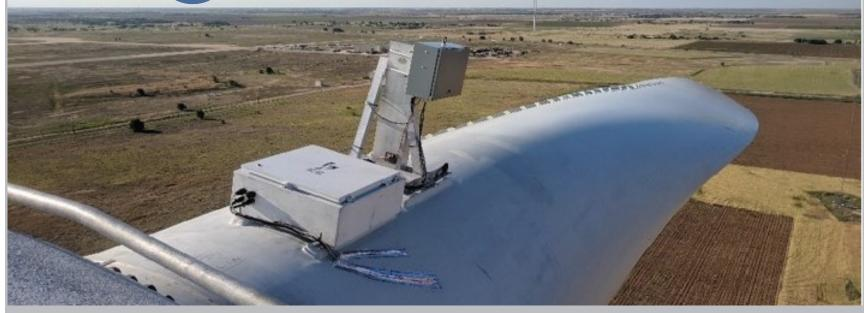
Wind turbine design engineers need to accurately predict how turbine blades behave under various operating conditions in order to optimize design and efficiency. **Boulder Imaging** (BI) provides the ability to **monitor**, **image** and **measure** how wind flows across blades while in motion. The results are used to continually optimize performance as turbines grow in size and energy output.
